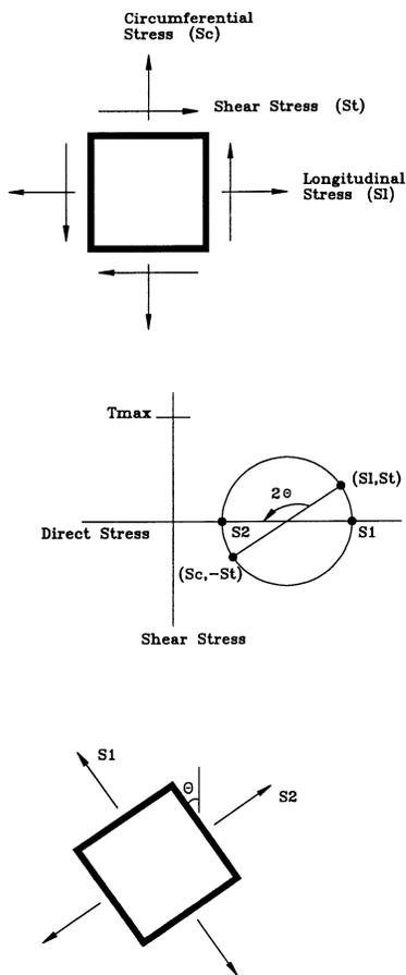
Since the radial stress is perpendicular to the rotated element and no shear term exists on the inside or outside surfaces of the pipe, the radial stress can be dropped on the zero-shear line of Mohr's Circle and serve as the principal stress in the third direction. **The maximum stress intensity is simply the greatest difference between two of these three principal stresses. This difference is also (by definition) twice the maximum shear stress on the element.**
