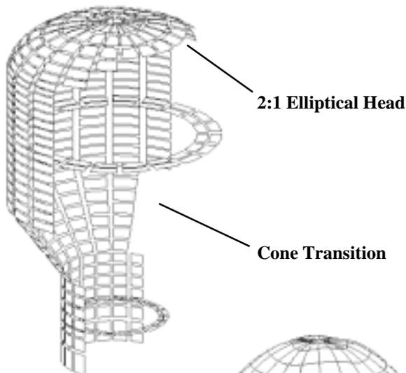
Exaggerated pressure displacements around stiffening ring. Highest pressure stresses occur at cone-cylinder transition.
