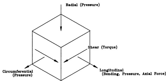
The local loads which make up these principal stresses are similar, if not identical, to those common in the piping codes. Mechanical loads in the axial, bending, and torsional directions and the pressure in the line are used with the corroded section modulus of the pipe to calculate local stresses at these four points through the pipe. The stresses calculated are as follows:
