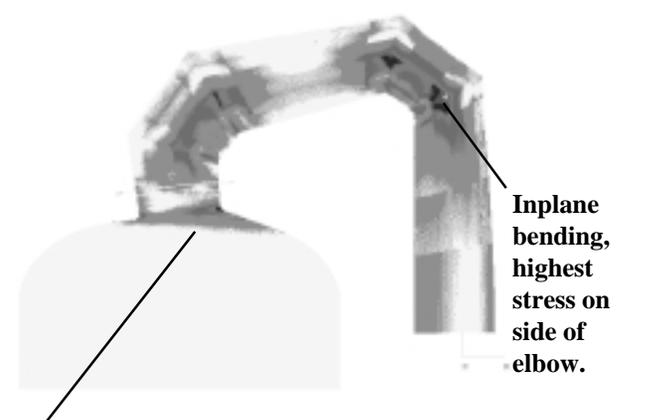
Stress pattern in head due to bending and shear is not symmetric as suggested by WRC 107.
