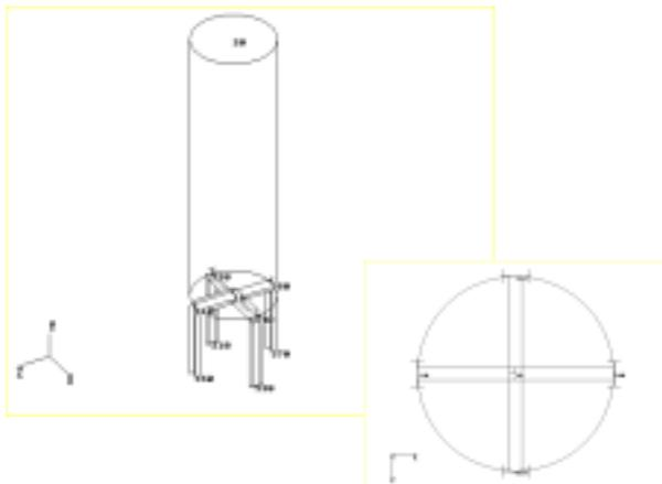
The initial review of the **CAESAR II** run verified that both the “wind only” case and the “weight only” case produced the correct (anticipated) loads. Now the combined load case results can be used with confidence.
