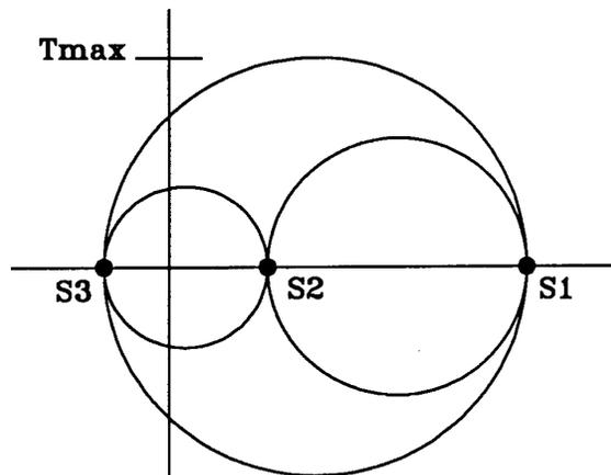
Again, this calculation is performed at four points through the pipe. The final step in producing the 3D maximum stress intensity listed in the CAESAR II report is to select the maximum of these four values at each node in the piping system.
